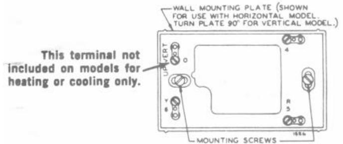
Fig. 1 — Wall Mounting Plate
