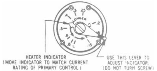
Fig. 4 — Adjustable Heater
