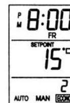
To see the ECONO programs, select the ECONO operating mode and press on PGM button successively to see programs 1 and 2 appear on the display. In ECONO mode, pressing on the ▲ or ▼ displays the temperature setting.
