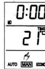
The active operation mode is the framed MAN mode, the setpoint is 20°C and the ambient temperature a displayed. If the display is different, maintain PGM button pressed down as RESET button is being pressed on and released. Then release PGM button.
