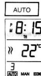
They are selected through the MODE button. On display, the active mode is framed. The frame moves on to the next mode each time the MODE button is pressed on.
