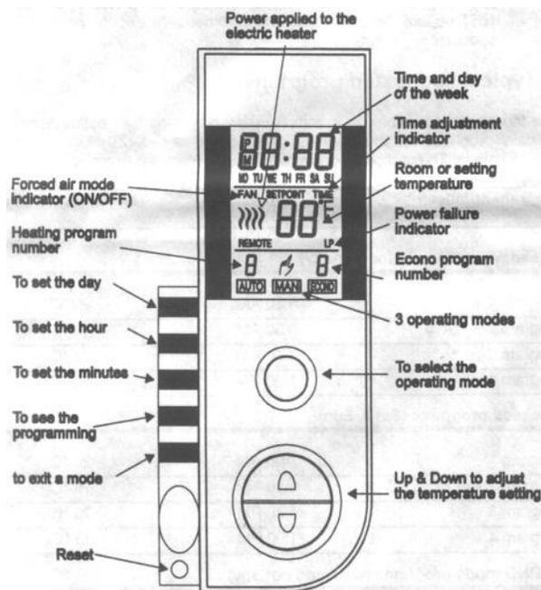
This thermostat is designed to be used with a self-protected heating system equipped with a thermal cut off and circuit breaker.
