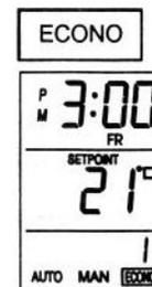
The ECONO mode has two (2) programs in which the day, the time, and the setpoint has to be programmed. For instance, this operating mode can be used for a cottage installation where the user goes only on weekends.
